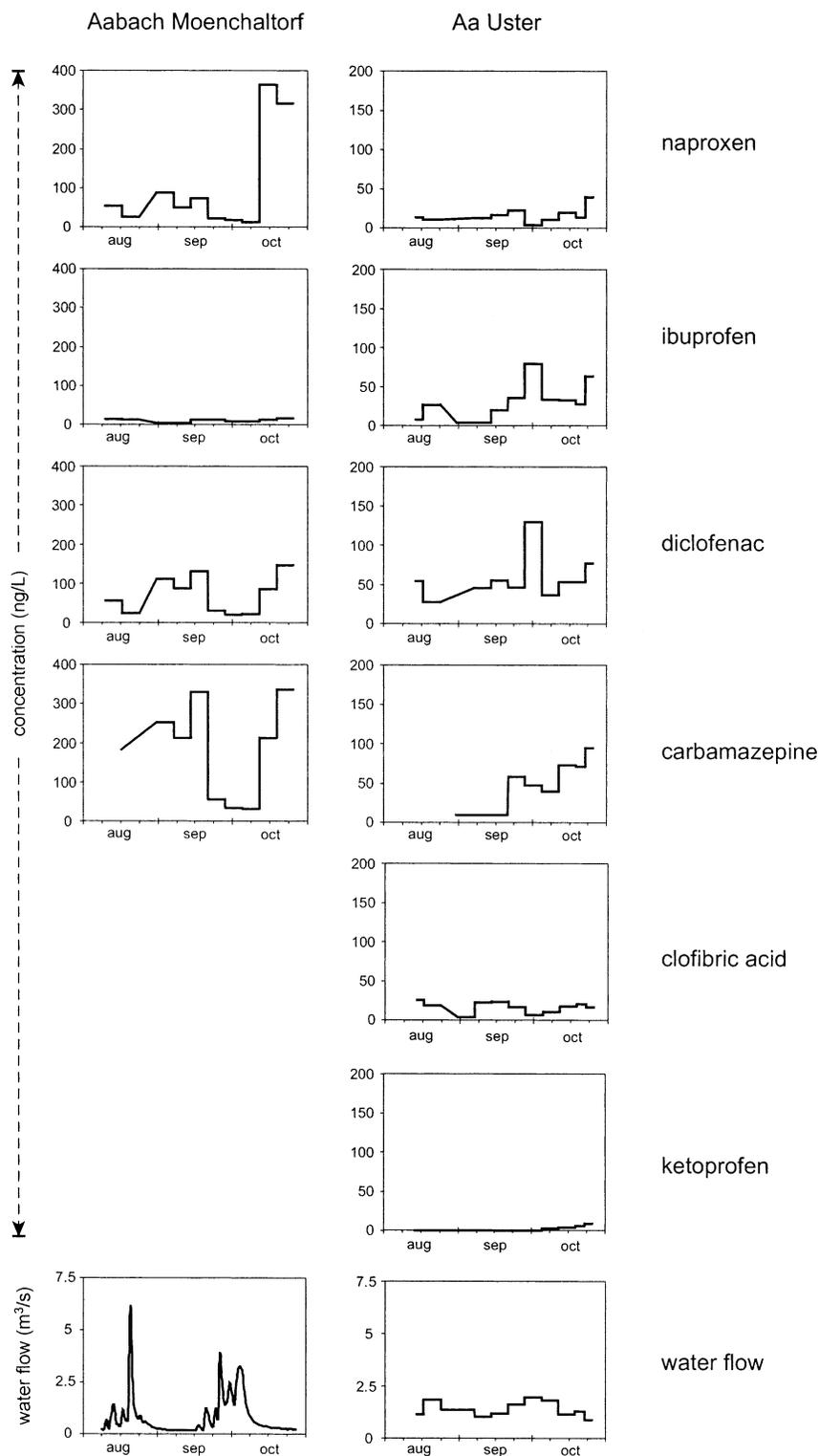
FIGURE 4. Continuous concentration measurements from August to October 1999 of the six pharmaceuticals and water flows in two rivers that receive wastewater from other four WWTPs.
