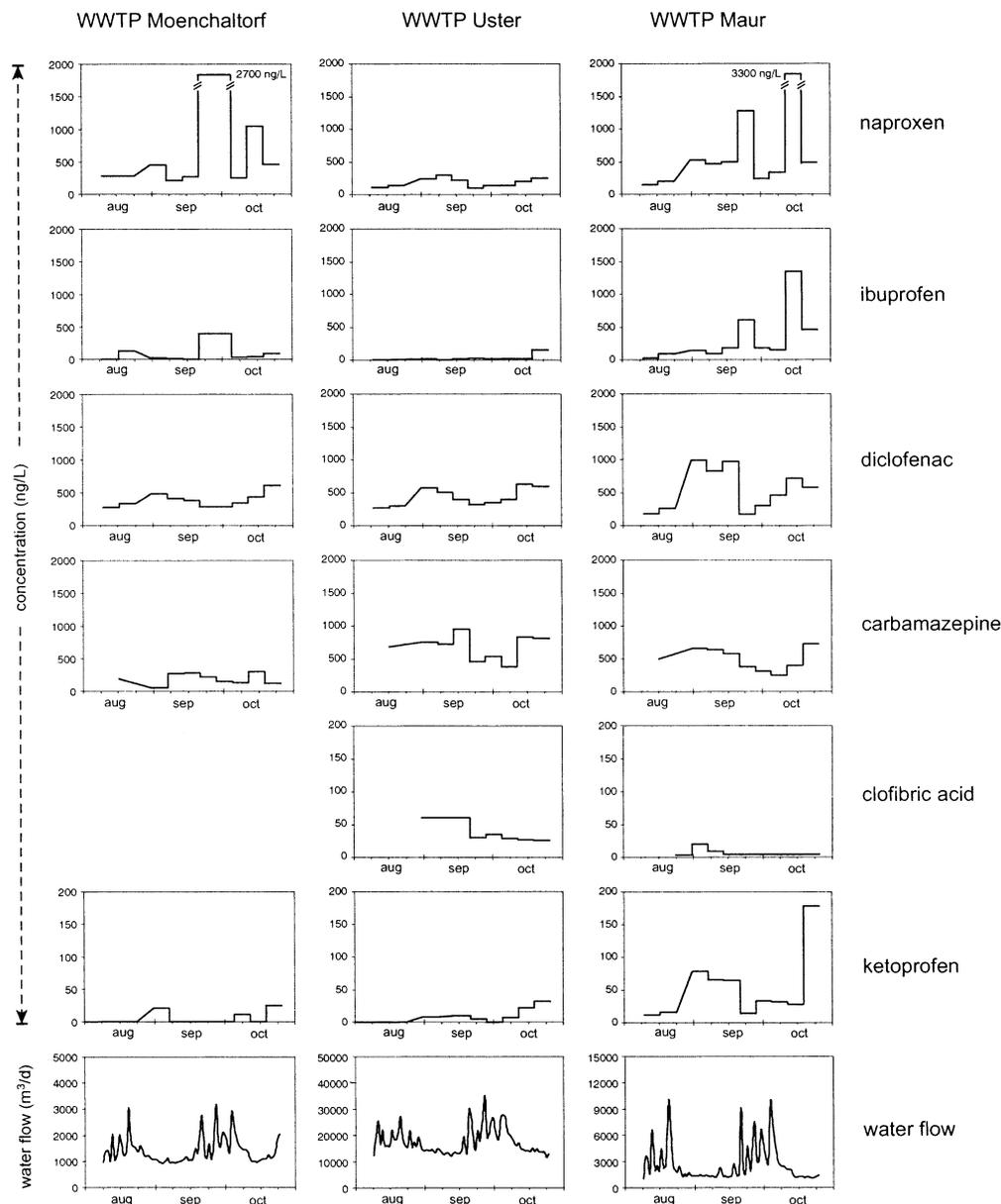
FIGURE 3. Continuous concentration measurements from August to October 1999 of the six pharmaceuticals and water flows in the effluents of three wastewater treatment plants directly discharging into the lake.
