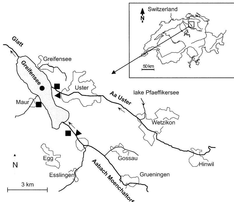
FIGURE 2. Sampling sites in the catchment area of Lake Greifensee: ■, effluents of wastewater treatment plants; ▲, sampling stations of the main tributaries; ●, water from the deepest point of the lake; polygons, village.
