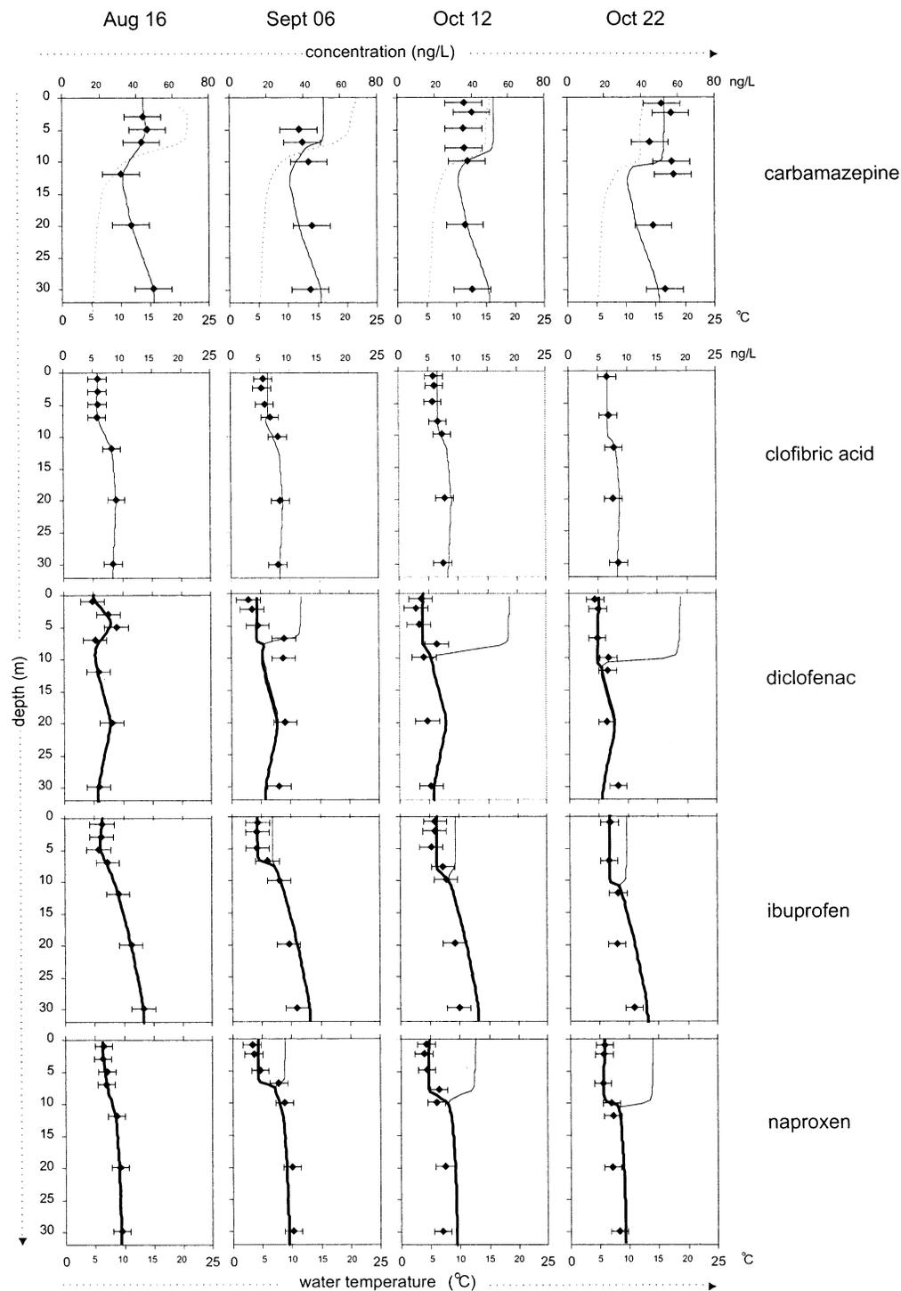
FIGURE 5. Monthly vertical concentration profiles of the six pharmaceuticals in Lake Greifensee:  $\blacklozenge$ , measured concentrations;  $\cdots$ , temperature profile; simulation results considering flushing as the sole elimination process (---) or considering flushing and another elimination process (—). (i) In the case of diclofenac, the second elimination process corresponds to the phototransformation; (ii) missing concentrations are due to analytical problems.
